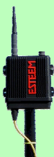
Model 195Es Series shown with outdoor pole mounting hardware and direct mount antenna.
